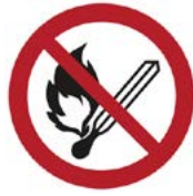
1 Prohibition sign: No open flame
